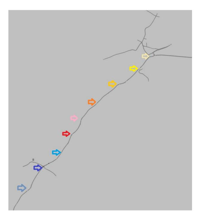
In terms of the speed readings these had been taken using a radar gun and L200 survey machine along the main A30 link. Readings had been taken both Westbound and Eastbound in both 40 mph and 60 mph sections at a variety of free flowing locations. The majority of the readings (195,771) applied to the 40 mph sections. A pivot table in EXCEL was used to create the speed flow curves and these were transferred as raw inputs in to VISSIM.
